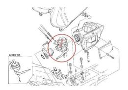
The RMV can be mounted under the seat, or behind the number plate. The more vertical the RMV the better and remember to avoid exhaust and engine components. For further information, see our easy step installation guide – Reservoir Positions, General. See third picture
