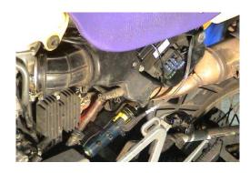
The Dispenser Assembly can be routed along the Swingarm and secured to the spindle using a Dispenser Plate & Clip. For further information see our easy step installation guide - <u>Dispenser Assemblies</u>, <u>General</u>. The nib should feed the rear sprocket between the 6 & 7 o'clock positions, with the cut face facing outwards.
